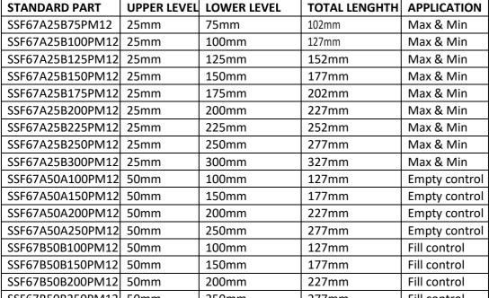
The SSF67 has been designed to give the user a long reach float switch with a number of switching options, to cater for a wide variety of system requirements. Manufactured in Stainless Steel 316L material, these switches are suitable for use in many aggressive liquids or hygienic applications.
