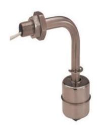
The CSSF24 seriesis acompact vertical float action switch that is horizontally mounted and designed to achieve reliable switching. Mounting isinthe side of the tank from the inside, so requires access to the inside of the tank.
